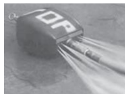
Examples of culvert cleaning nozzles appropriate for Isolator Row PLUS maintenance. (These are not StormTech products).
